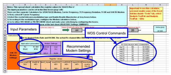
Figure 6. OOK Modem Parameter Calculation
