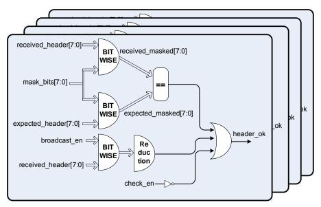
Figure 8. Receive Header Filter
