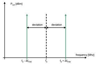
Figure 4. FSK Modulation
