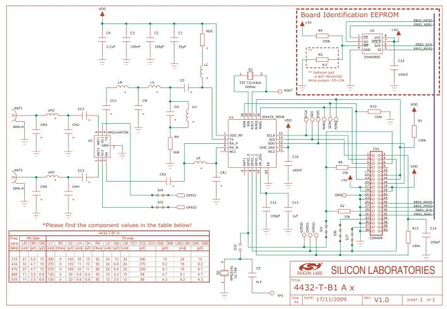
Figure 3. Antenna Diversity Si4432 Testcard Schematic
