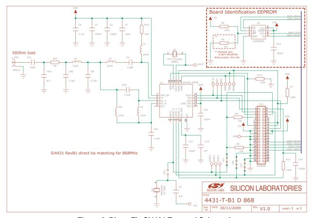
Figure 2. Direct Tie Si4431 Testcard Schematic
